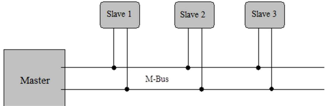
**Master to Slave =>** The transfer of bits from master to slave is accomplished by means of voltage level shifts.
